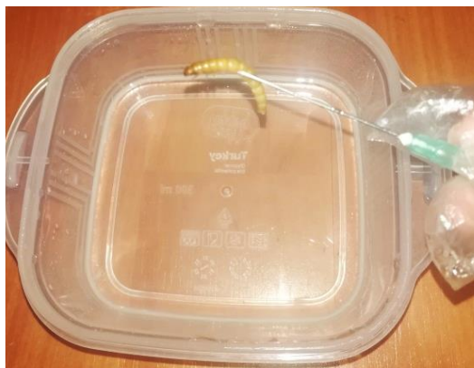
Figure 2. Stage of immersion of Tenebrio molitor larva in epoxy environment
