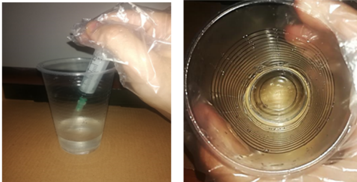
Figure 1. The mixture which prepared using resin and hardener
